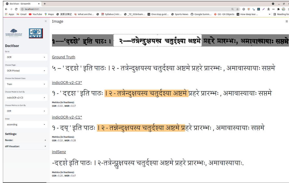
Fig. 8: OCR interface in DocVisor depicting the image-text alignment by leveraging the attention mechanism from the OCR architecture of Agam et. al. [5]. Refer to Sec. 5. Notice that there are multiple (2) attention OCR models along with non-OCR models that can be loaded in the OCR layout that allows the user to compare line level results of multiple models simultaneously.
